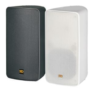
The RD 108 is a highly weather-resistant, single 8" 2-way full range loudspeaker, the body is made of engineering plastic injection molding. fitted with one 8" mid-woofer and one 1" HF driver. The system conforms to IP46 international standard.
